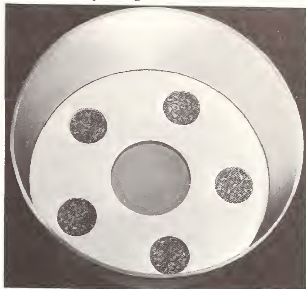
FIGURE 5.—A multichoice food preference chamber with samples from one untreated and four treated bins of grain sorghum.
